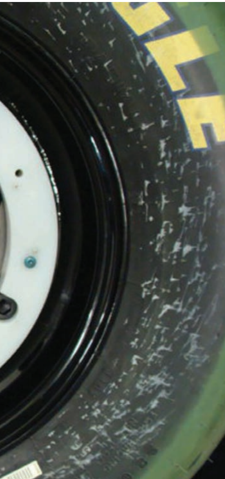
LEFT: Patented wheel force transducers are groundbreaking technology for side force measurement. The white ring on the wheel contains electronics and wireless transmitters. There are embedded strain gauges on the wheel hub. Wireless receivers mounted in the wind tunnel transmit data back to Test SLATE
